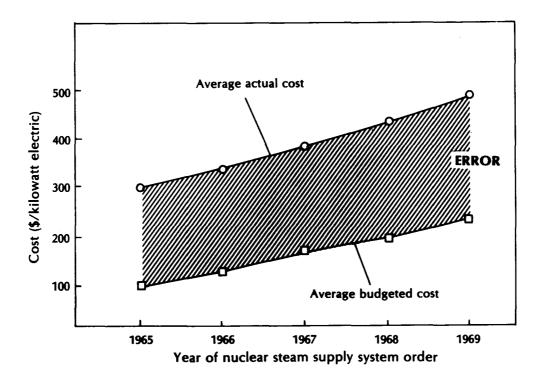
Gross misestimation of reactor costs has troubled the nuclear industry. The bottom line represents estimated costs of a reactor ordered in a given year, and the top line the actual costs ordered or expected (1973 dollars).
